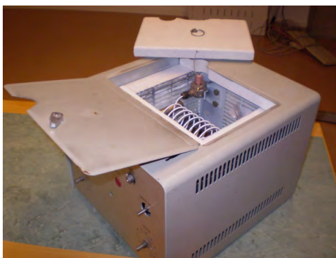
Figure 3.2: The old gas chromatograph Søren Jensen used for the discovery (own photo).
